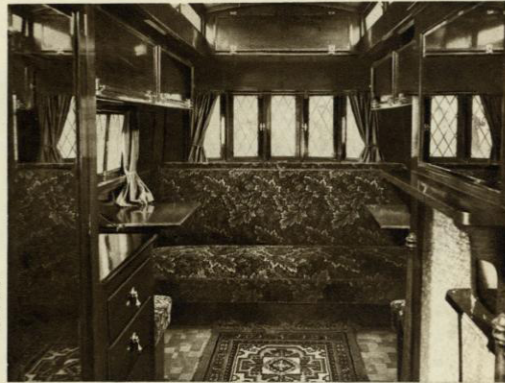
Interior Eccles Living Van showing the settee which turns over to form a double-bed, also a stove and overmantel. Behind is a large airing cupboard. Many of these Vans are fitted with a coil range.
